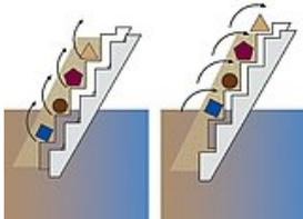
Phase 2 + 3: The complete screenings carpet is lifted and transported by rotation of the moveable laminae.
