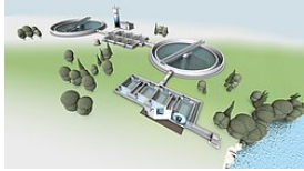
Fourth treatment stage: Typical process with HUBER Disc Filter RotaFilt® as downstream polishing filter: (1) PAC dosing, (2) Contact basin, (3) Sedimentation tank, (4) Polishing filter with HUBER Disc Filter RotaFilt®
