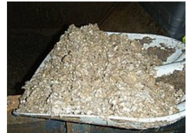
Screenings with no free water
