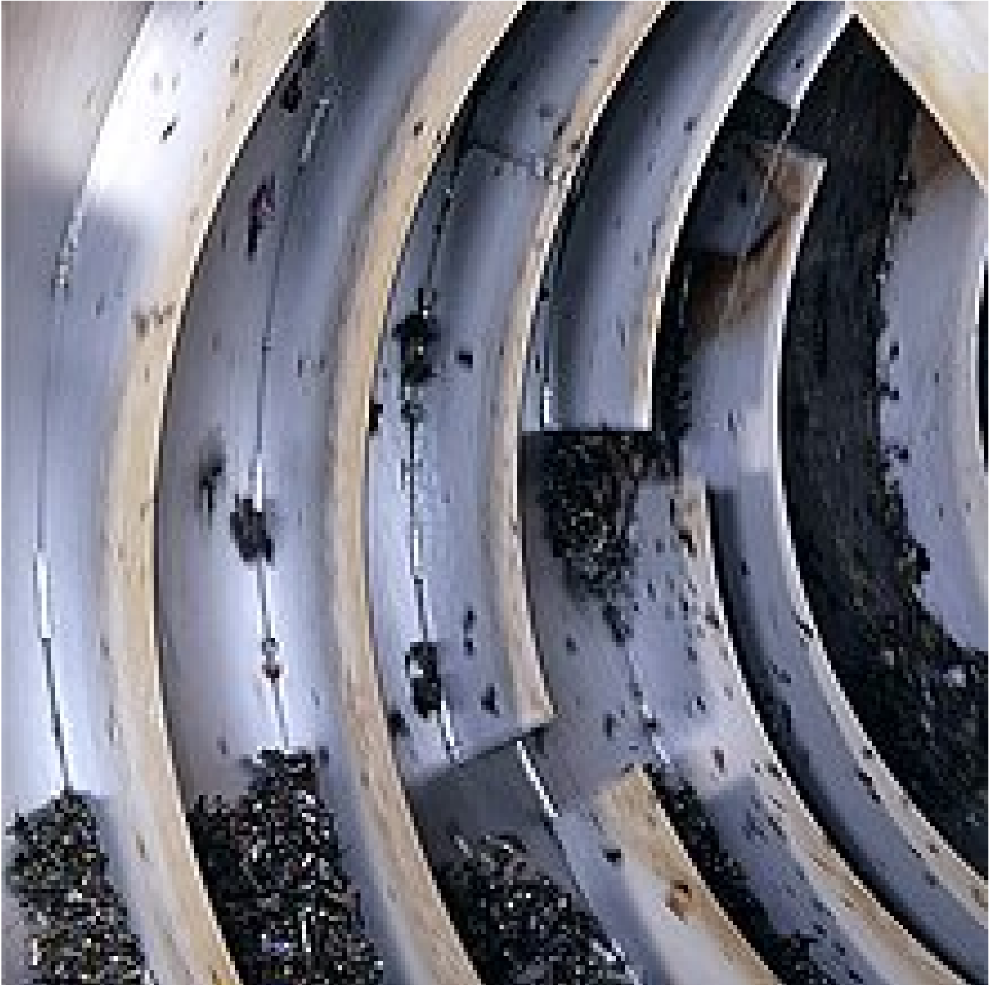
HUBER Sludge Acceptance Plant RoFAS separating coarse material
