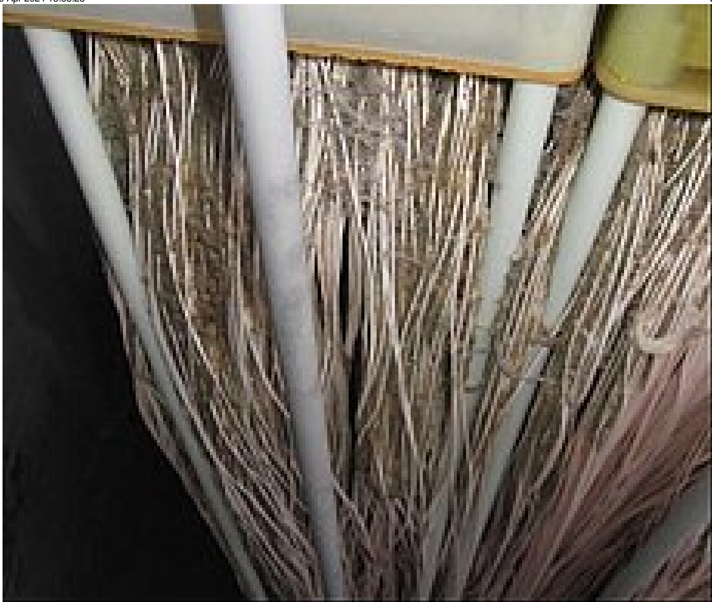
Insufficient pre-treatment of wastewater leads to clogging of fibre membranes
