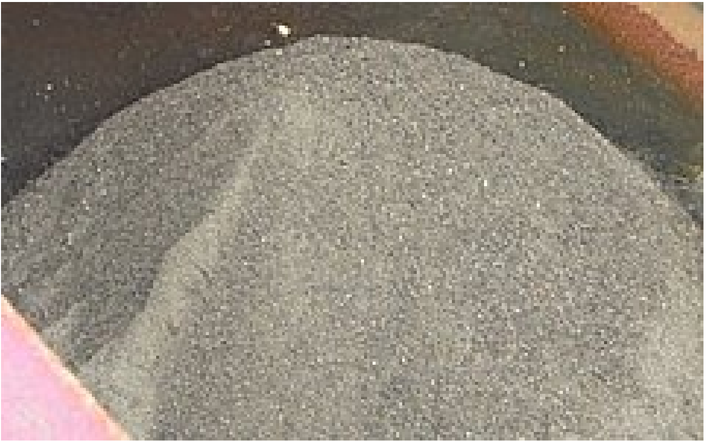
Figure 3 – Washed grit, prevented from accumulating in the digester
