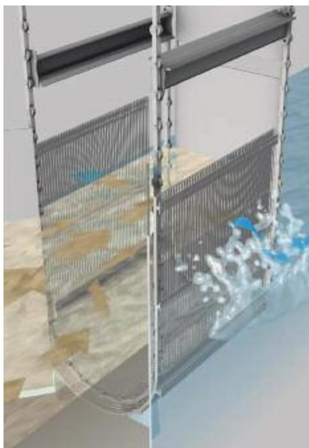
*The deflection of the flow improves the filter effect of the bar rack and increases solids separation efficiency.*
