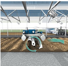
A double shovel is ploughing through the sludge bed and turning the sludge as the machine is moving through the greenhouse
