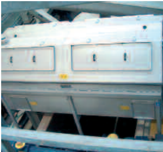
Micro-Screen ROTAMAT® RoMesh in a tank
