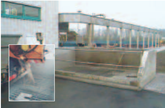
Acceptance tank with bar grate and integrated vertical dosing screw
