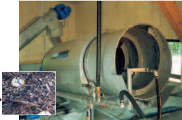
ROTAMAT® Wash Drum for washout and separation of all coarse material > 10 mm
