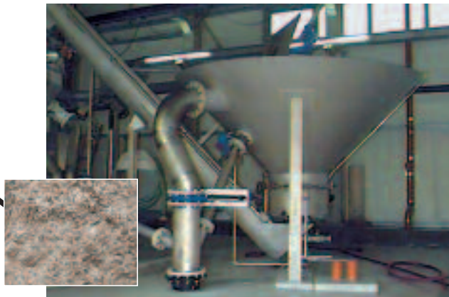
Washed grit from COANDA Grit Washer with < 3% loss on ignition, particle size up to 10 mm, DR > 90%
