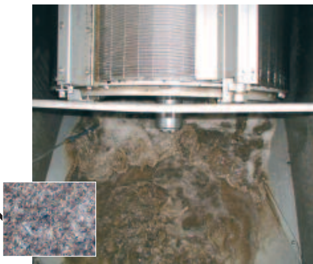
ROTAMAT® fine screen for 1 mm screening and dewatering of organic material (approx. 30 % DR)
