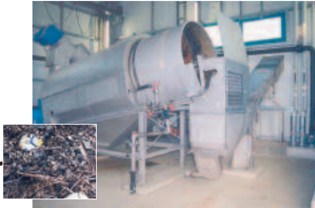
ROTAMAT® Wash Drum for washout and separation of all coarse material > 10 mm
