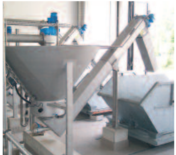
Reduced disposal costs and improved hygienic conditions with the COANDA Grit Washing Plant
