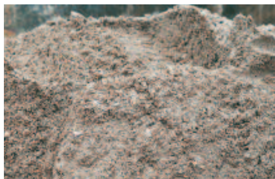
Washed grit removed at a wastewater treatment plant
