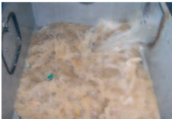
High turbulence in the launder tank during impeller operation
