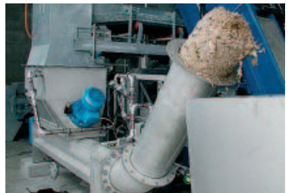
Well washed and virtually odorless screenings from a WAP/SL, compacted to 50 % DS
