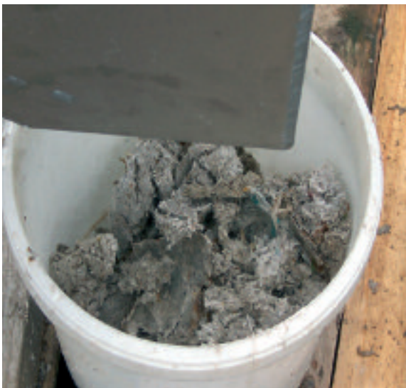
Screening of municipal wastewater with a high content of fibres (in particular toilet paper)
