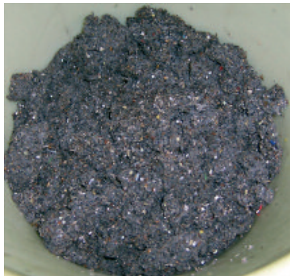
The Pipestrainer removes very fine screenings (such as hairs) after a preceding coarse screen
