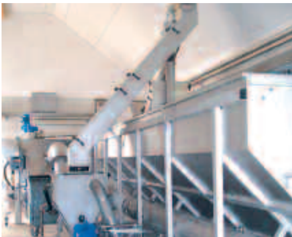
Intensive washing of screenings in a WAP/SL Wash Press subsequent to a Complete Plant Ro 5
