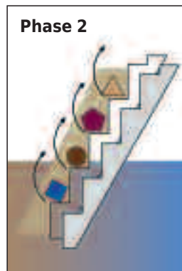
Phase 2 The complete screenings carpet is lifted and transported by rotation of the moveable lamella unit.
