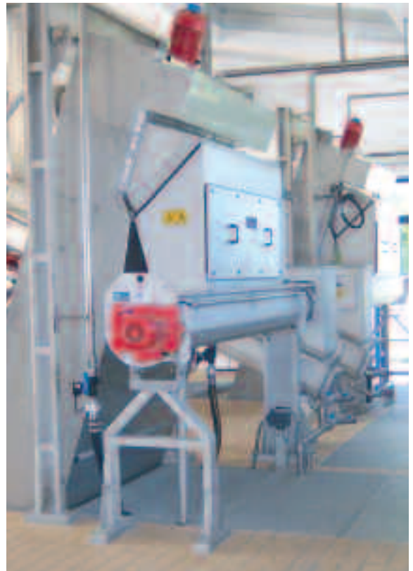
Side view of an enclosed STEP SCREEN SSV® for odour-free screenings discharge
